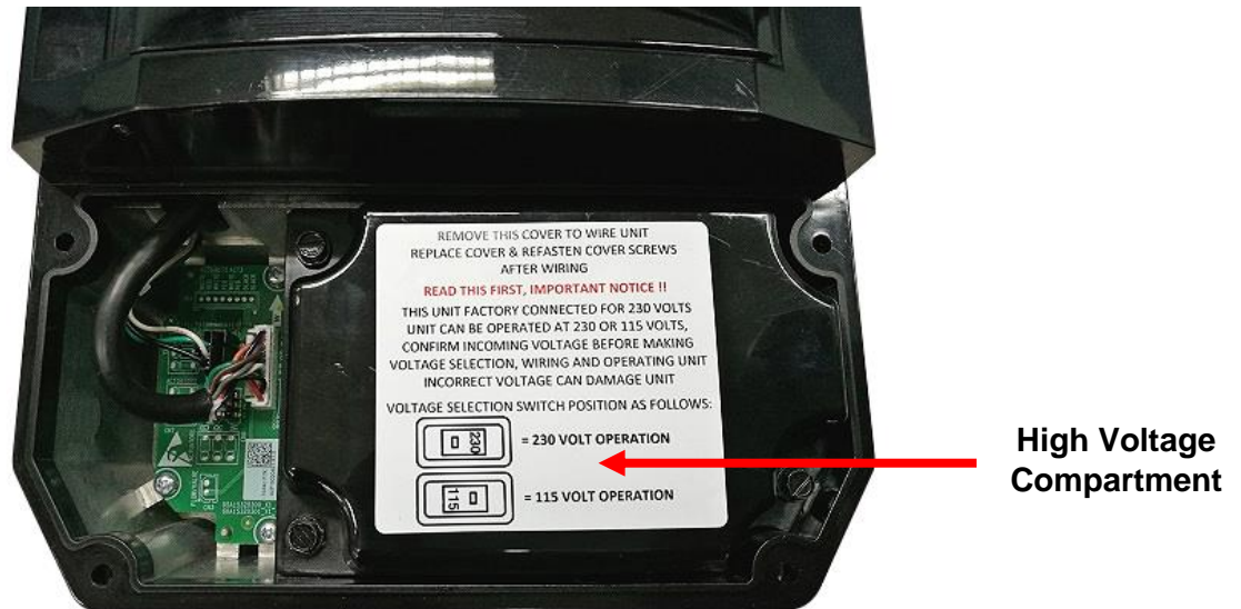
Figure 1 – High Voltage Compartment
