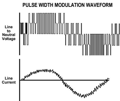
Figure 1 PWM Waveform
