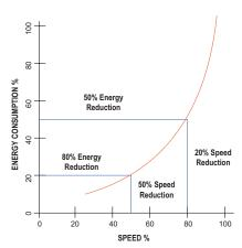
What if this were a 30 hp fan running at 90% of its speed?  $0.9 \times 0.9 \times 0.9 = 73\%$ Multiply 73% with 30 hp = consumption of 21.9 hp
