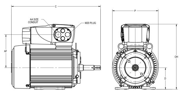
Unique assembly dimesions below. All other dimesions per NEMA
