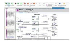
CT Scope provides real-time monitoring of up to 8 channels to verify the drive configuration is operating as expected Connect software enables developers, system integrators and installation contractors to focus on application requirements when setting parameters, not on acquiring deep knowledge of the ID300's integrated drive.
