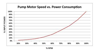
This graph shows the large increase in energy consumption when running the pump and motor at high speeds. Slowing the pump and motor speed saves significant energy dollars, similar to better automobile gas mileage when driving 40 mph versus 70 mph.
