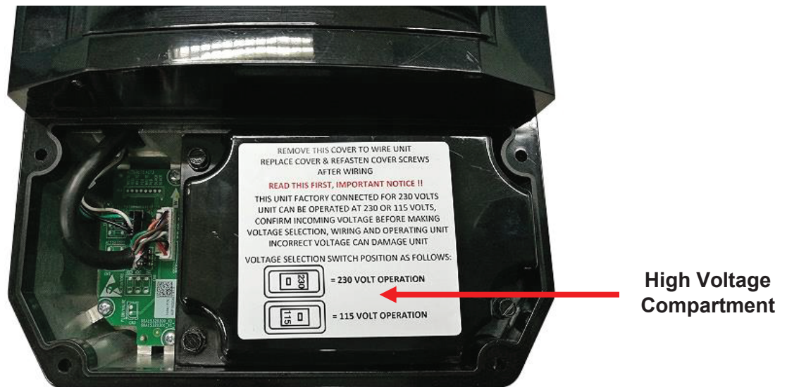
Figure 1 – High Voltage Compartment
