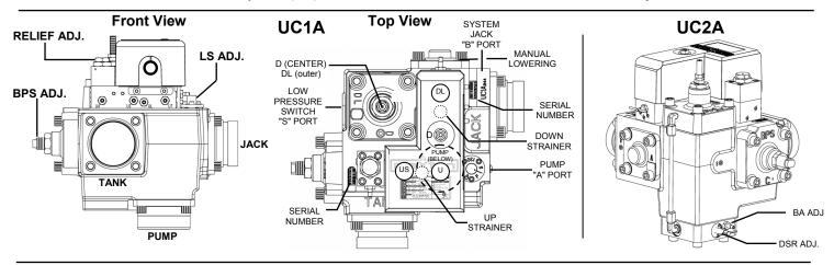
ATTENTION: All Maxton Valves **MUST** be installed with the solenoids in the upright (vertical) position. Prior to 2012 the sleeve and baseplate were an integral part of coil operation. 2012 to current the C-Frame and Bracket are an integral part of coil operation.
