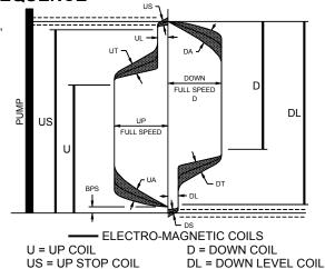
CAUTION: On Wye - Delta Up Start do not energize U and US Coils until motor is running on Delta
