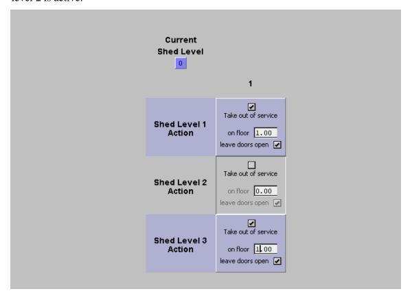
20. To activate load shedding, right click the Current Shed Level box and select activate shedding. Under "Override Value" choose the shed level (1, 2 or 3). You may also set a duration for the shed level if desired.
