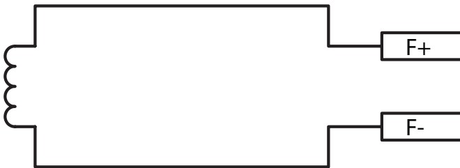
Figure 12 Field Power Output Connections
